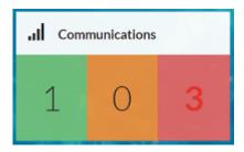
This tile gives access to the communication statistics table. It displays the radio level and the number of measurements retrieved, for example, which are key indicators for a proper functioning of a measurement chain. This list is exportable. Values colour changes from black to orange then to red depending on the statistics.
