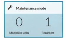
A monitored unit or a recorder can be set into maintenance mode in MySirius (with a deadline and reason) during corrective intervention on the monitored equipment or the device used for monitoring. Select the mnitored unit or the recorder and click on MAINTENANCE. This operation stops alerts and measurements sending to MySirius. Monitored units and recorders undergoing maintenance are identified by a yellow / black colour in the OPERATION / ADMINISTRATION tab.
