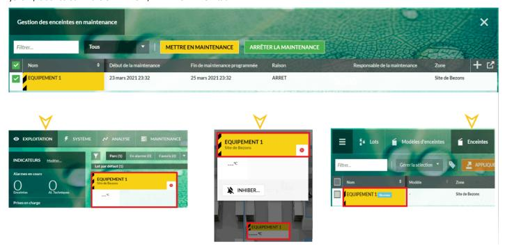
Setting back a unit to OPERATIONAL mode is done by clicking on the STOP MAINTENANCE MODE button.
